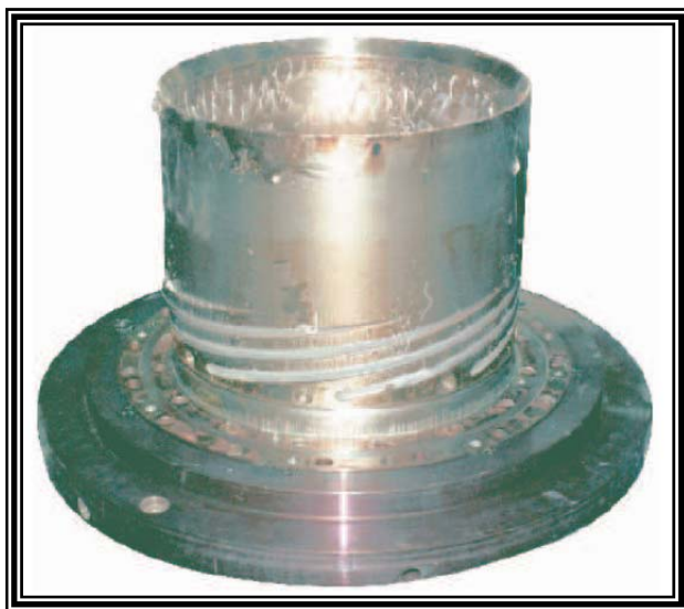
Part of a blown film die prior to cleaning
