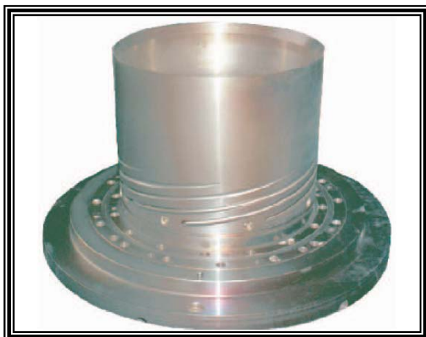
Part of a blown film die after cleaning
